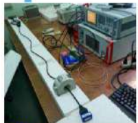
BCI test environment (ISO 11452-4: 2011)
